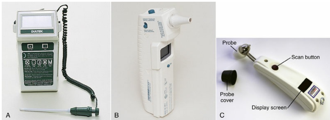
FIG. 3-7 A, Electronic thermometer. B, Tympanic thermometer. C, Temporal artery thermometer. (B from Seidel et al., 2011; C from Bonewit-West, 2012.)
